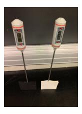
6. Place the pockets with the thermometers directly under the lamp so that both receive equal amounts of light. The lamp should be pointing straight down.
